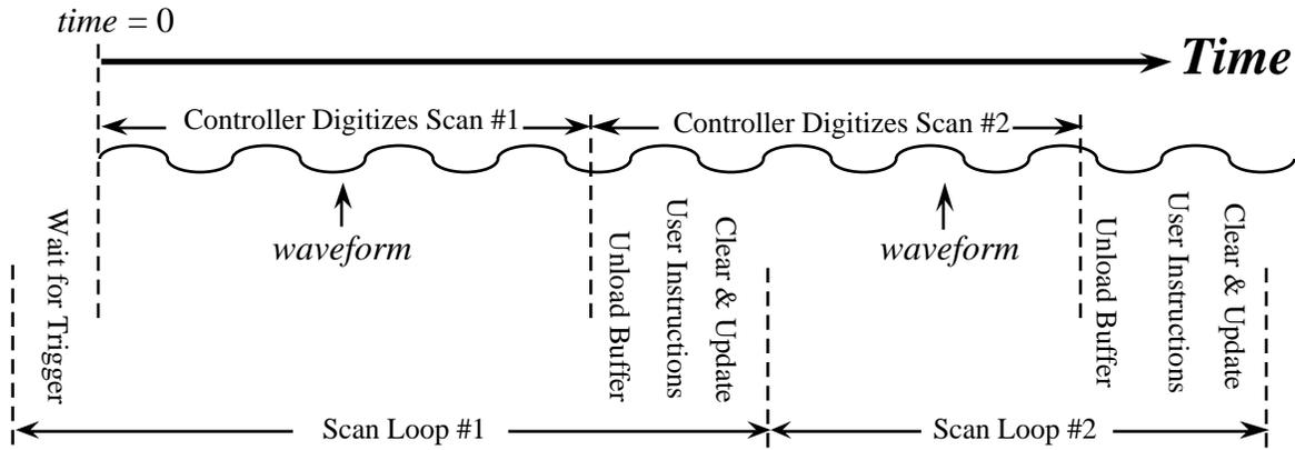
Strip chart instruments are triggered once at the beginning of all scans. This is in contrast to Oscilloscope instruments that are triggered separately at the beginning of each scan.
